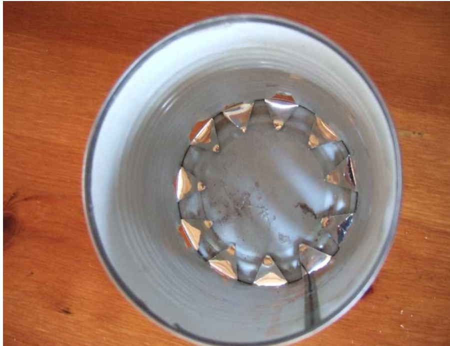
This month we build a simple green wood chip burner from a tomato can.
