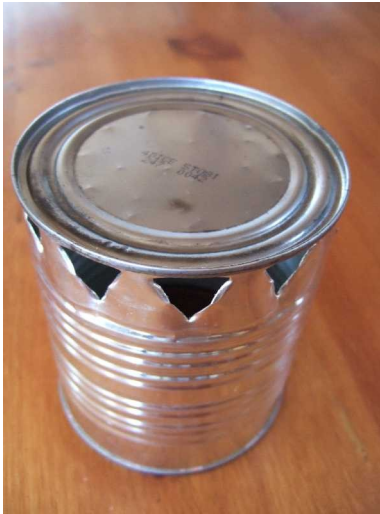
The burner can, inverted to show base holes
