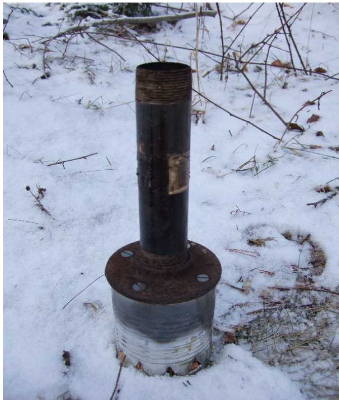
The Hermes stove. Note the heat stratification and lack of smoke
